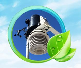
The Montford Middle School WeatherSTEM Unit is an integration of weather sensors, the data gathered and stored by the sensors, and a dynamic display of the data in a website that showcases the current weather, weather forecasts, data mining tools, lessons & activities, weather notifications, and more!
